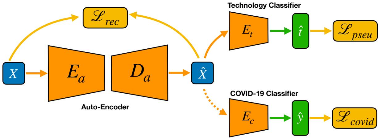
Fig. 1. The architecture of our proposed *PrepNet* model consists of three main modules: (i) an auto-encoder that acts as a CT cross-dataset homogenizer; (ii) a multi CT-technology classifier; and (iii) a COVID-19 binary classifier. The auto-encoder and the multi CT technology classifier are trained adversarially. The binary COVID-19 classifier is independently trained using the auto-encoder’s output.
